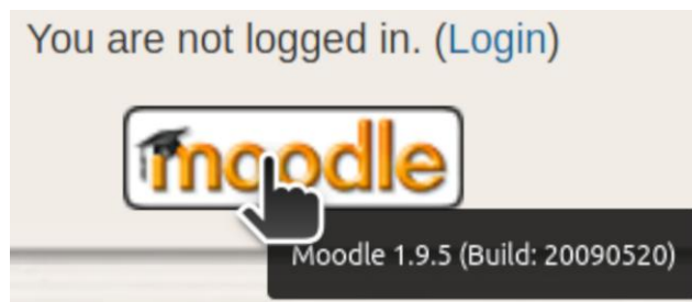
Figure 2 Moodle 1.9.5 version revealed with build number to an unauthenticated user (screenshot from actual production site – 2025).
